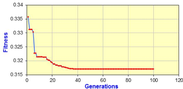
Fig. 3: Genetic Algorithm Graph for Grinding X12M by Cn46.CV1.G.V400x40x203x35m/s
