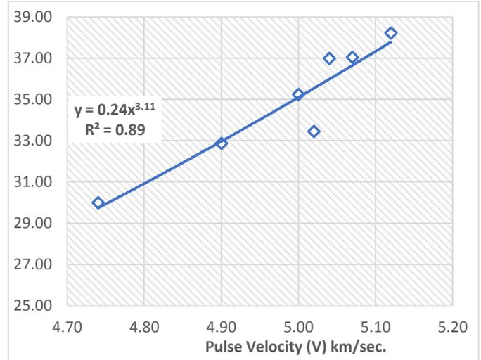
Fig. 13:  $E_c$  vs. V
