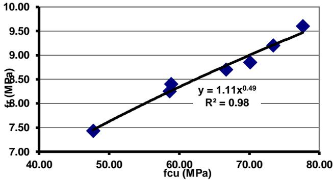
Fig. 8:  $f_r$  vs.  $f_{cu}$
