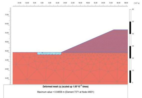
Fig. 5: Filling of 2m foundation pit with reinforced soil
