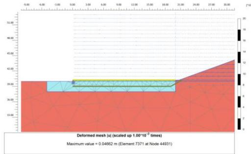
Fig. 6: Filling of reinforced soil along with the placing of facing and geogrid
