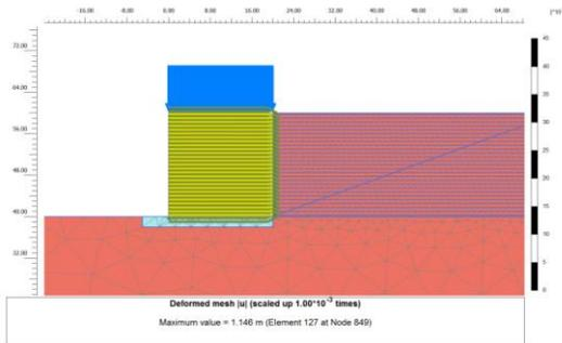
Fig. 8: 20m full height MSE wall with surcharge load on top of it
