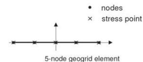
Fig. 1: Position of nodes and stress points in geogrid elements
