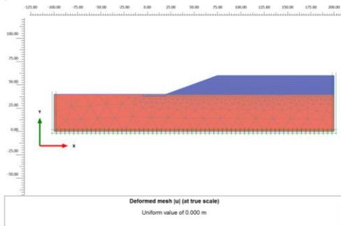
Fig. 3: The existing ground of initial phase in staged construction mode
