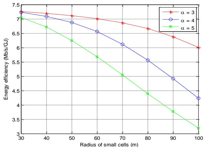
Fig. 5: Energy Efficiency of the Star Configuration for Different Values of Path Loss Coefficient.
