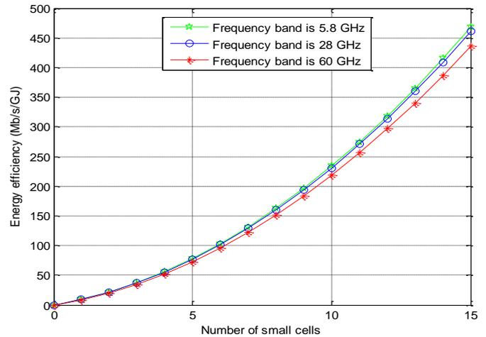
Fig. 4: Energy Efficiency of the Mesh Configuration for Different Frequency Bands for 15 Nodes Only.
