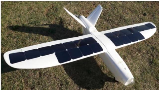
Fig. 14: Completed Aircraft with Integrated Solar Cells.
