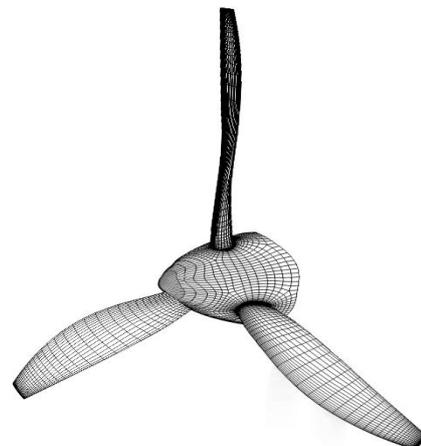
Fig. 2: Computational mesh (coarse mesh is shown)
