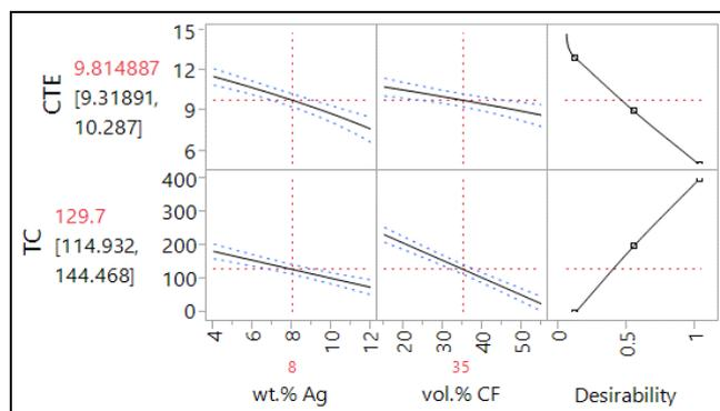
**Fig. 7:** Predicted profiler for CTE and TC of Cu-Ag/CF composites.
