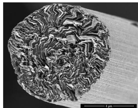
Fig. 1: The microstructure of XN-100 carbon fibre.
