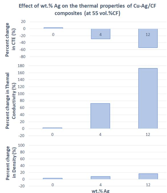
**Fig. 9:** Thermal performance of Cu-Ag/CF composites relative to the normal Cu-CF composites.
