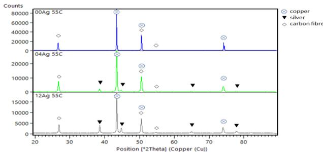
**Fig. 3:** The XRD pattern of the Cu-Ag/CF composites at 55 vol.% carbon fibres.
