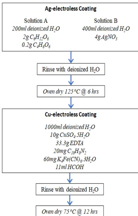
Fig 3: The electroless coating of carbon fibres.
