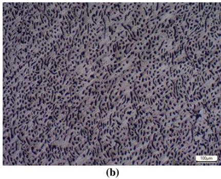
**Fig. 6:** The distribution of the carbon fibres in the direction (a) perpendicular to the pressing direction and (b) parallel to the pressing direction.
