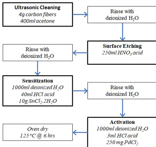
Fig 2: The surface treatments of carbon fibres.
