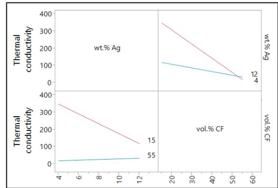
**Fig. 8:** Interaction profiles of the thermal conductivity of Cu-Ag/CF composites.
