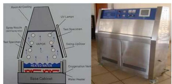
**Fig. 4:** UV-weathering chamber for sunlight simulation
