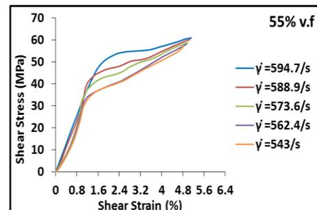
**Fig. 6:** Stress-Strain curves for Random Fiber E Glass-Epoxy-Composite with different Volume-Fraction
