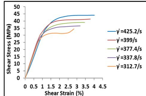
**Fig. 5:** Stress-Strain Curves of Epoxy
