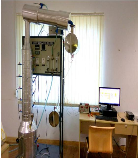
Fig. 5: Real time distillation column
