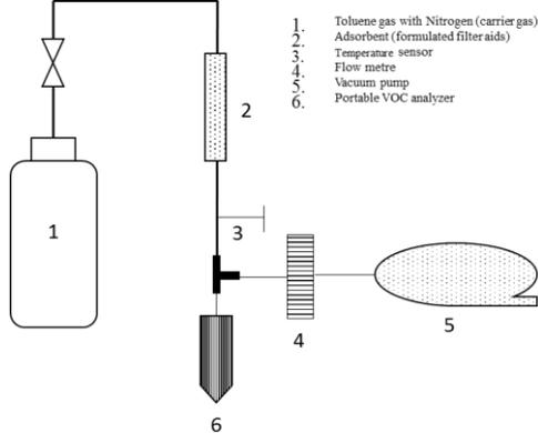
**Figure 1.** A schematic diagram of the experimental set-up to study VOC adsorption over formulated filter aids
