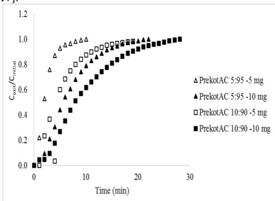
**Figure 3.** The effect of amount of adsorbent on breakthrough curve of toluene gas over formulated filter aids
