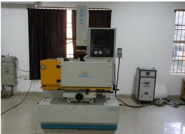
Figure 1: Electric Discharge Machine
