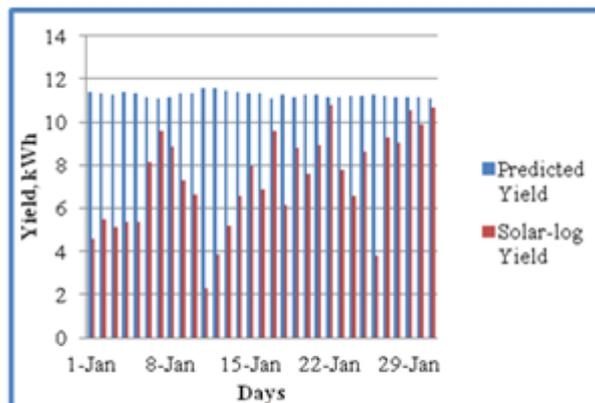
Fig. 6: Comparison between the calculated  $Y_f$  and the actual  $Y_f$  for January 2018.
