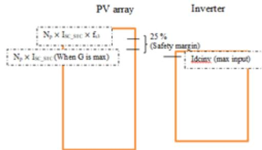
Fig. 5: Matching of PV array current to inverter current.
