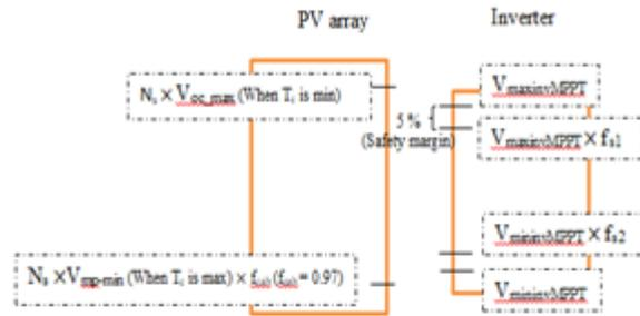
Fig. 4: Matching of PV array voltage to inverter voltage.
