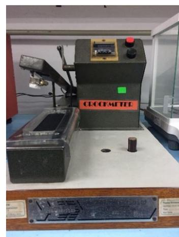
Figure 3: The crockmeter machine for rubbing/crocking test
