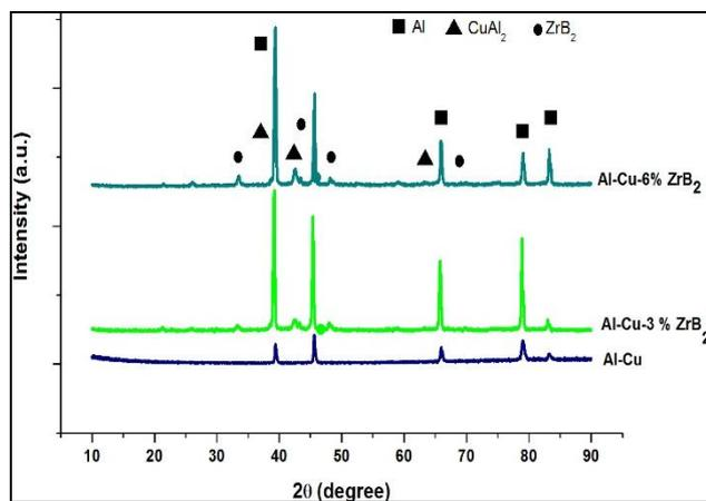
Fig. 2: X-Ray Diffraction patterns of Al-Cu reinforced with 3 wt.% and 6 wt.%  $ZrB_2$  *in-situ* composites
