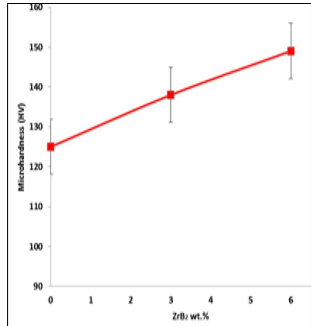
Fig. 6: Evolution of microhardness of *in situ* ZrB<sub>2</sub> reinforced composites via the weight fractions of ZrB<sub>2</sub> reinforcement
