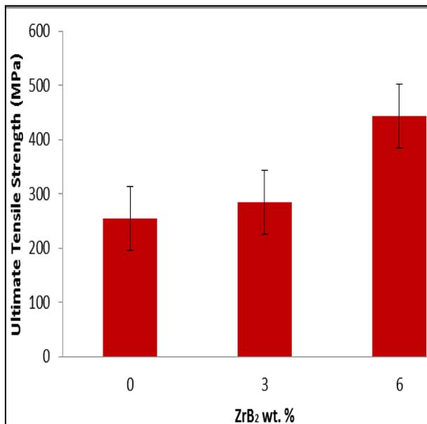
Fig. 4: Effect of weight percentage of ZrB<sub>2</sub> on ultimate tensile strength of Al-Cu MMCs
