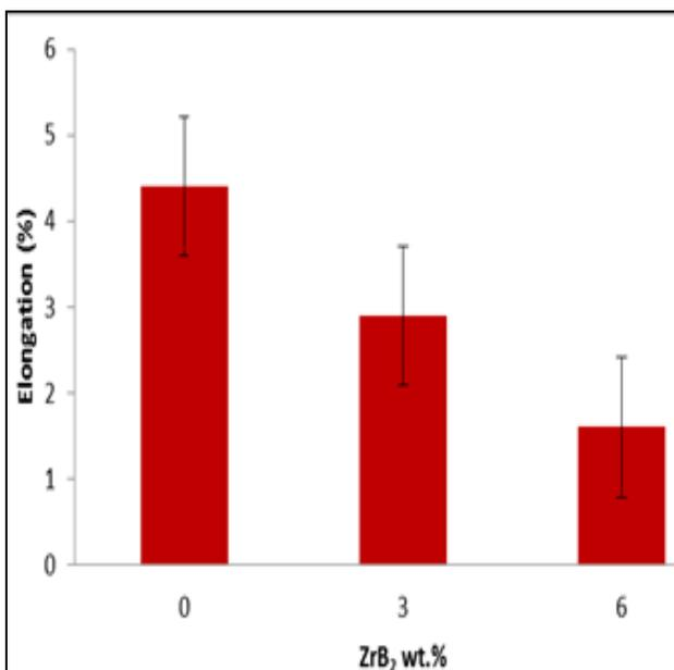
Fig. 5: Effect of weight percentage of ZrB<sub>2</sub> on elongation of Al-Cu MMCs
