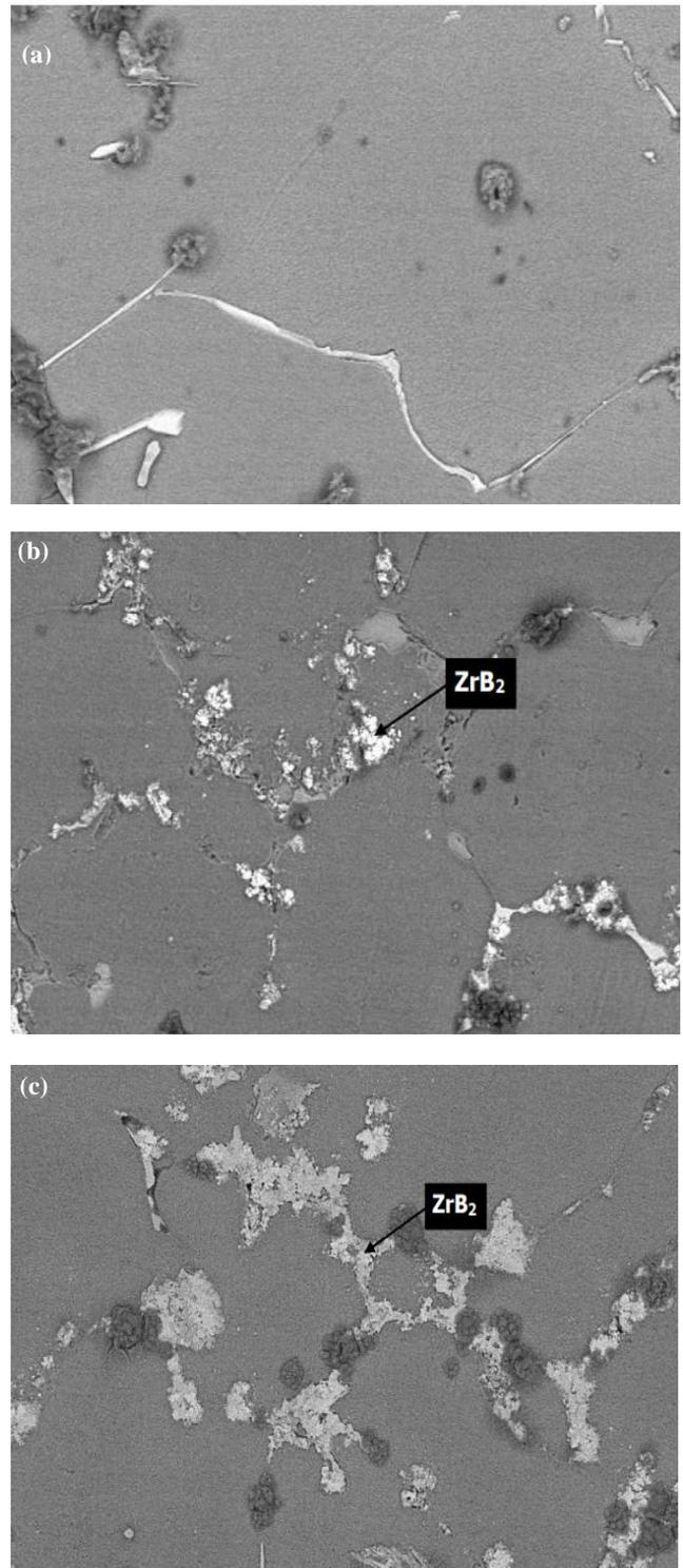
Fig. 3: FESEM images of Al-Cu *in situ* composites containing (a) 0 wt. %  $ZrB_2$ , (b) 3 wt. %  $ZrB_2$  and (c) 6 wt. %  $ZrB_2$
