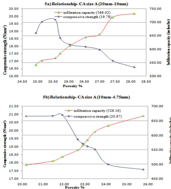
Fig. 5: Relationship between Compressive Strength, Porosity and Infiltration Capacity.
