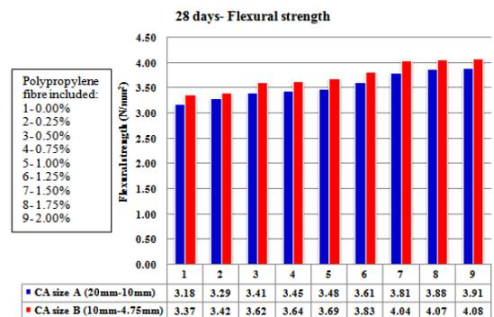
Fig. 3:Flexural Strength of Fibre Included Pervious Concrete.
