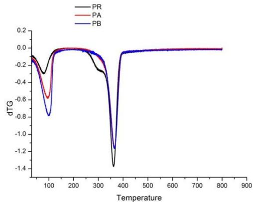
Fig. 4: Thermal graph of PR, PA, PB (a) TGA graph (b) DTG graph
