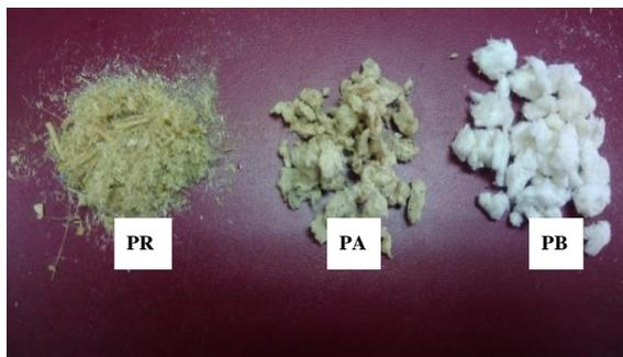
Fig. 1: (PR) Raw PALF (PA) Alkali Treatment PALF (PB) Alkali + Bleaching Treatment PALF
