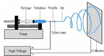
Fig. 2: Electrospinning machine set up
