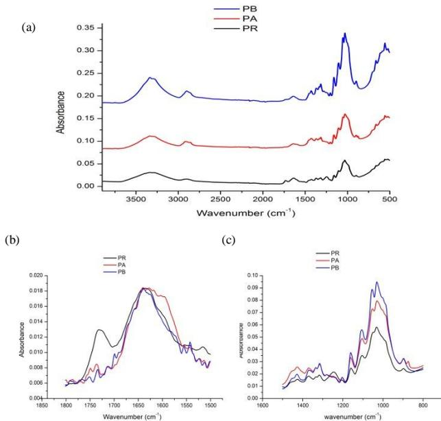
Fig. 3: (a) FTIR spectra of PR, PA and PB (b) zoom in at  $1500\text{-}1800\text{cm}^{-1}$  (c) zoom in at  $800\text{-}1500\text{cm}^{-1}$
