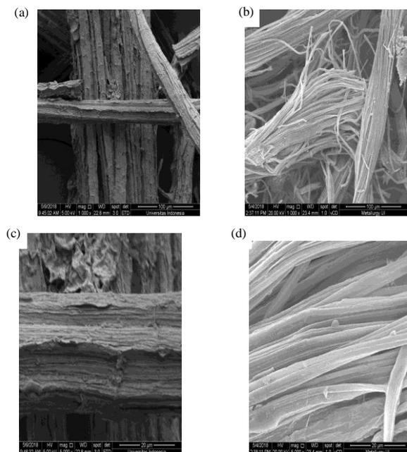
Fig. 6: Surface morphology result of (a) PR (1K x mag), (b) PR (5K x mag) (c) PB (1K x mag) (d) (5K x mag)
