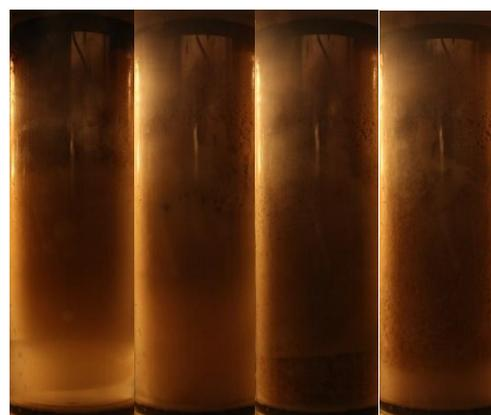
Fig. 7: Crude oil B emulsion behavior pictures of before (above) and after (bottom) with produced ASP ratio PW: ASPW (80:20), Pressure = 4.5bar, Temperature =30°C, water cut = 55%
