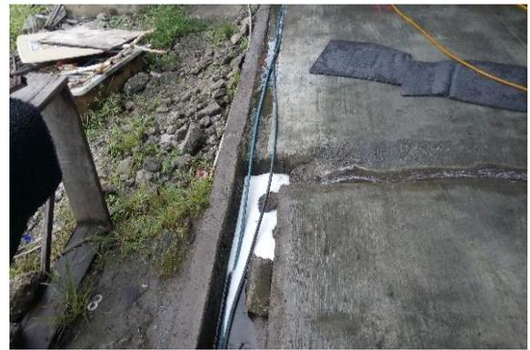
Fig. 2: Collecting sample car wash environmental water at outlet drainage of car wash wastewater
