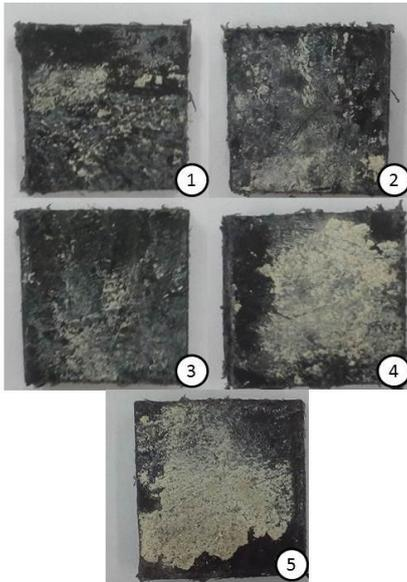
**Fig. 3:** The appears of the form samples with a layer of hardened cement mixture (after the production process) after the first treatment with the appropriate mixtures
