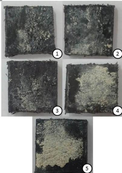
**Fig. 4:** The appears of the form samples with a layer of hardened cement mixture (after the production process) after the second treatment with the appropriate mixtures
