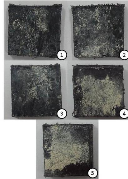
**Fig.5:** The appears of the form samples with a layer of hardened cement mixture (after the production process) after the third treatment with the appropriate mixtures
