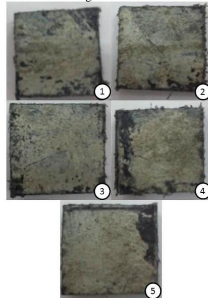
Fig. 2: Initial appears of specimens of the form with a layer of hardened cement mixture (after the production process)
