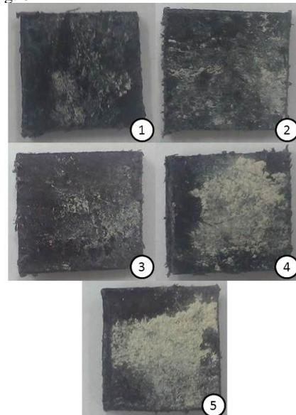
**Fig. 6:** The appears of the form samples with a layer of hardened cement mixture (after the production process) after the fourth treatment with the appropriate mixtures
