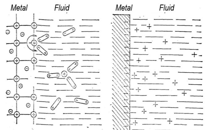
Fig. 2. The scheme of occurrence of the difference of electric potential
