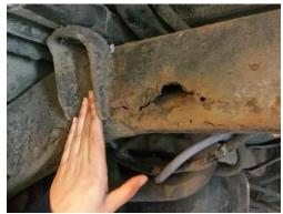
Fig. 3: Damaged frame
