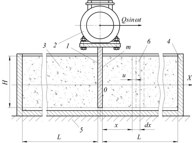
**Fig. 1:** The design diagram of the interaction of a deep compacter with a concrete mix in the form: 1 - a flat vertical plate; 2 - vibration exciter; 3 - concrete mix; 4 - form; 5 - base; 6 - selected item.
