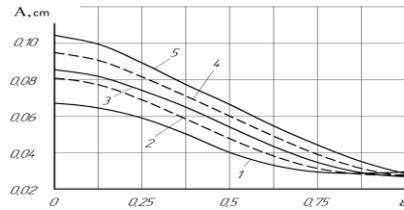
**Fig. 3:** Changes in the amplitude of vibrations of a deep-surface planar vibration compactor interacting with a compacted medium of different consistency depending on the relative density of the concrete mix at  $L = 60$  cm: 1 - with a draft of 3.5 - 4 cm; 2 - when the stiffness of the mixture  $S = 30$  s; 3 - at  $S = 60$  s; 4 - at  $S = 90$  s; 5 - at  $S = 120$  s
