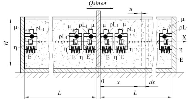
**Fig. 2:** Rheological model of a concrete medium compacted in a form.
