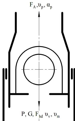
Fig. 3. The calculation scheme of the forcing valve's work: the start of lifting after the plunger has passed the upper "dead" point
