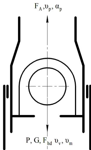
Fig. 2. The calculation scheme of the forcing valve's work: lowering when the plunger is removed from the lower "dead" point
