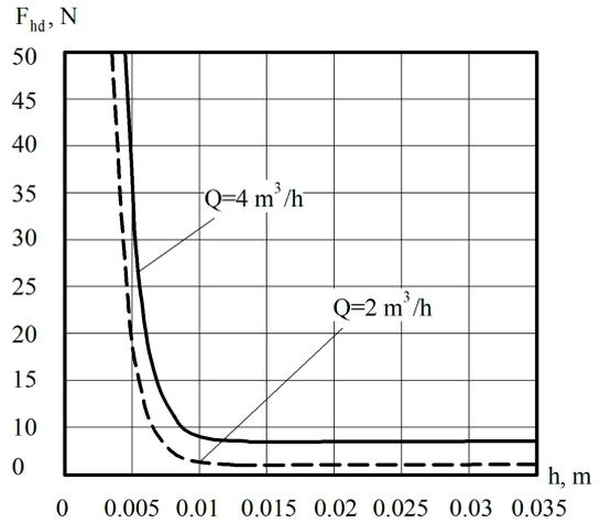
Fig. 6. Dependence of the force of the hydrodynamic flow pressure on the ball on the lifting height of the ball over the seat for the different value of the mortar flow with the mobility of 10 cm
