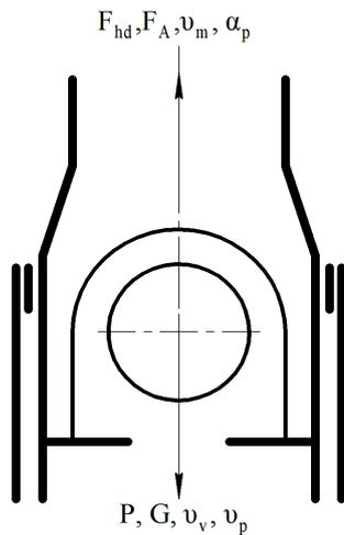
Fig. 1. The calculation scheme of the forcing valve's work: the beginning of the ball lowering at the moment of the plunger approaching to the bottom of the "dead" point
