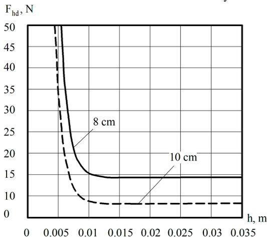
Fig. 5. Dependence of the force of the hydrodynamic flow pressure on a ball on the lifting height of the ball over the seat for mortars of various mobility at constant feed
