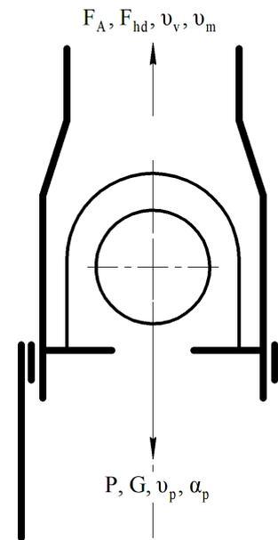
Fig. 4. Operational scheme of the forcing valve: lifting at the distance from the upper "dead" point
