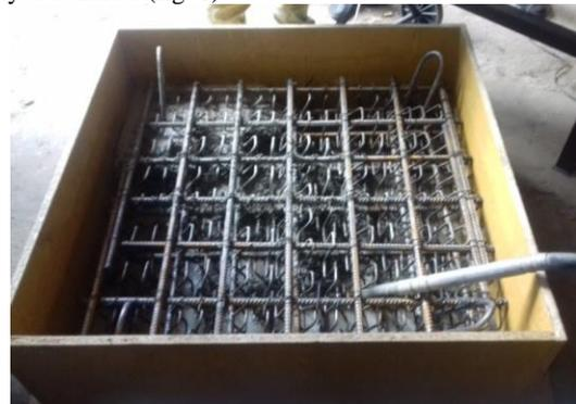
**Fig. 1:** Formwork with an enclosed frame, prepared for concreting plates P1 and P2
