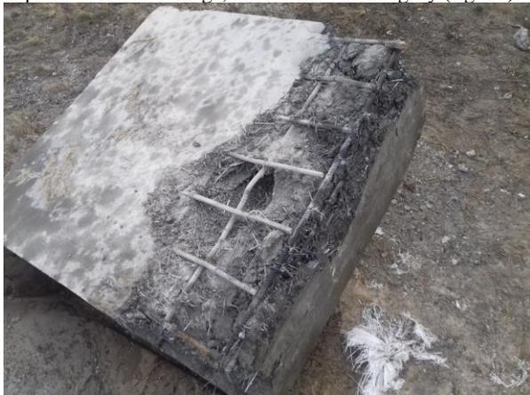
Fig. 10: Hitting the plate P-2 with a firing pin thickness of 120 mm
