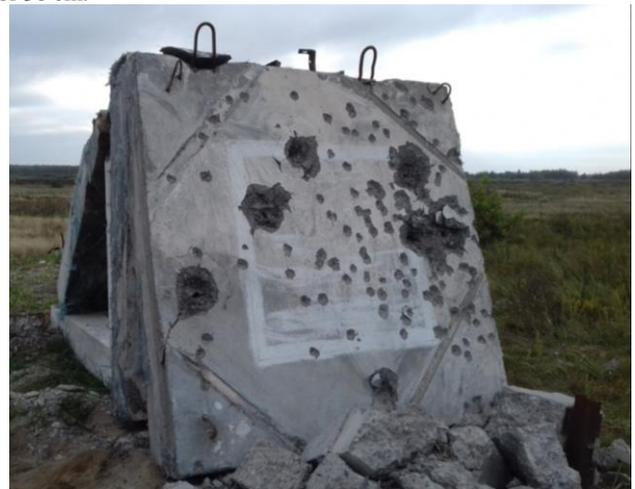
Fig. 11: Hitting PSH-2 plate with a 30 mm firing pin
