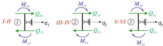
Fig. 2: Calculation schemes of the column nodes
