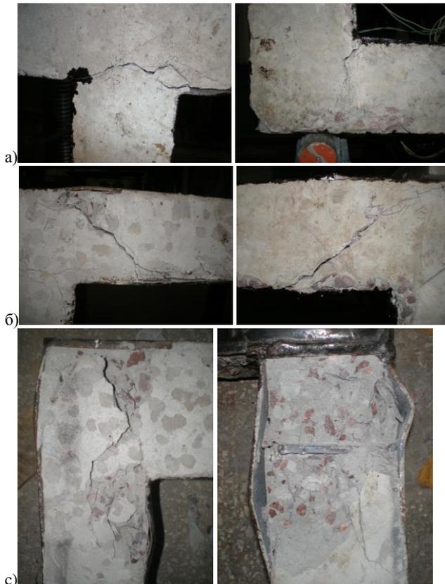
**Fig. 10:** The nature of the destruction of the test elements' joints during the physical experiment: a - the structure SRCE-1-1, tested for bending; b - the structure SRCE-1-2, tested for bending; c - the structure SRCE-1-3, tested for compression.
