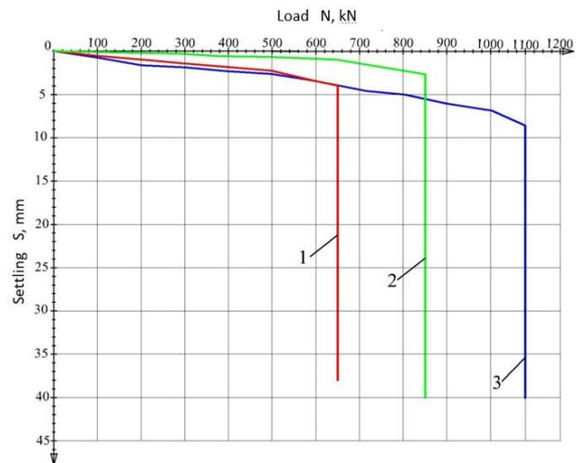
**Fig. 11:** Charts of dependence of piles settling on vertical static loads: 1 - unreinforced soil-cement pile; 2 - VRSCP №2; 3 - VRSCP №3
