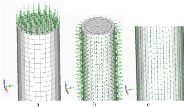
Fig. 2: Schemes of loads to the model of the pile: a) vertical useful to the pile head; b) lateral compression by the soil; c) the load of lateral friction
