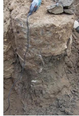
**Fig. 5:** Destruction of the unreinforced the vibroreinforced soil-cement pile on the material.
