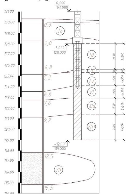
Fig. 4: The position of the vibroreinforced soil-cement pile on the engineering-geological section and its division into high-altitude sections
