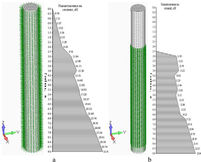
Fig. 3: The distribution of the height of the piles a) the side compression of the pile by the soil; b) frictional forces between the lateral surfaces of the pile and the soil during its compression
