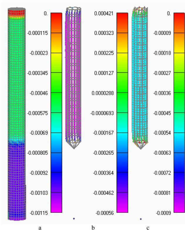
**Fig. 13:** Distribution of relative longitudinal deformations on the surface of the vibroreinforced soil-cement pile (a) and in the reinforcing bar rods of the general (b) and separately compression (c)
