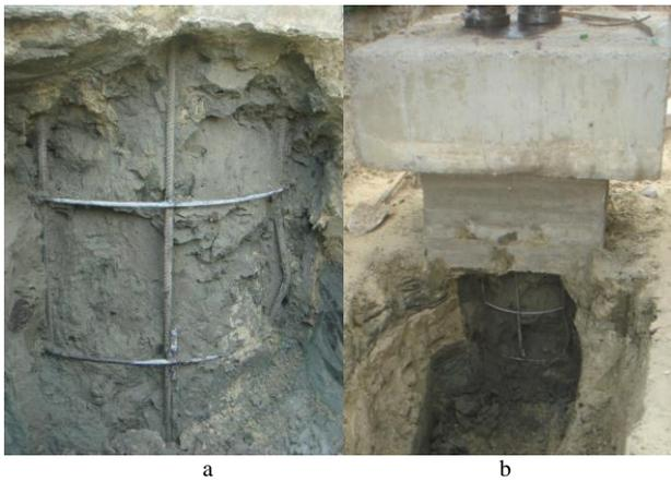
**Fig. 7:** Reinforcement frame cleared from the protective layer of vibro-reinforced soil-cement pile after the test: a - study of the destruction of the frame after the test; б - the general view of piles at digging out.
