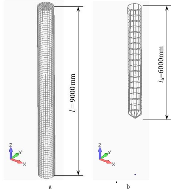
**Fig. 1:** Model of a the vibroreinforced soil-cement pile (a) and a reinforcing frame (b), broken into finite elements of solid type in the form of hexahedrons Hex Mesh
