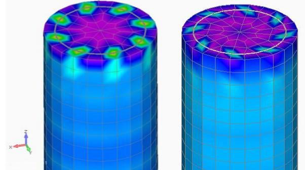
**Fig. 14:** Redistribution of effort between reinforcing rods and the vibroreinforced soil-cement pile in the section of the pile
