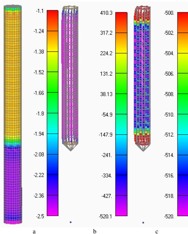
**Fig. 12:** Distribution of stresses normal to the longitudinal axis in MPa on the surface of the vibroreinforced soil-cement pile (a), in the reinforcing bar rods of the frame (b) and separately only the gripping (c)
