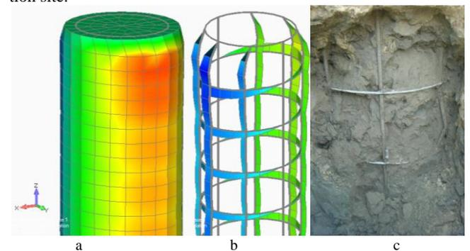
**Fig. 15:** Concentration of stresses near the head of the pile: a) on the surface of the model; b) in reinforcing rods; c) during a full-scale experiment
