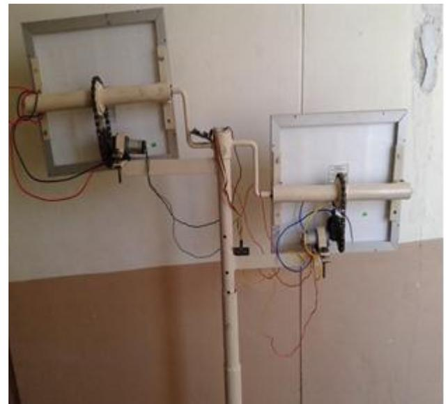
Fig. 11: Time Lapse Based Single Axis MPP Tracking System for Solar Tree back view
