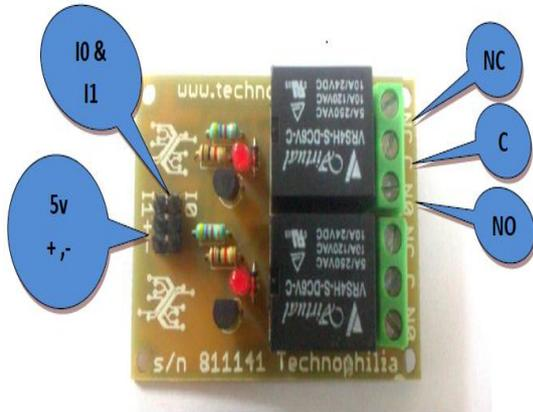
Fig. 3: Relay Circuit
