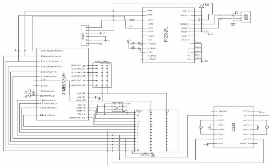
Fig. 7: IC2 schematic diagrams of time lapse solar tracking system
