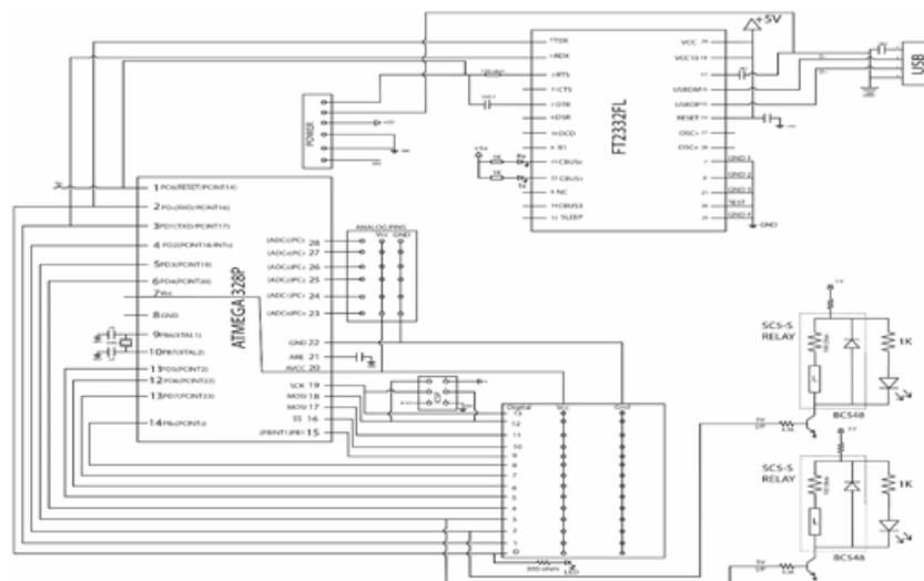
Fig. 8: Main relay schematic diagrams of time lapse solar tracking system
