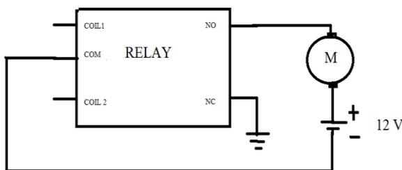
Fig.5. Relay Connection
