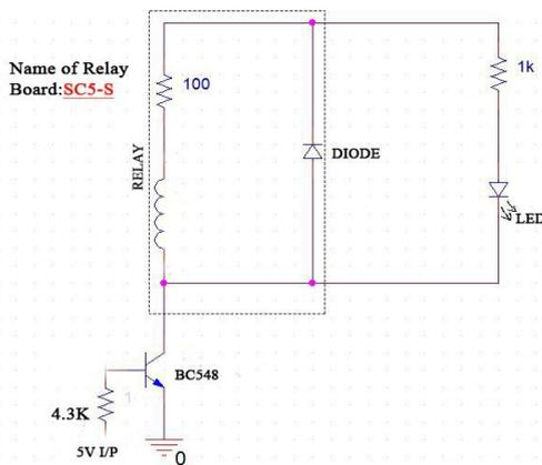
Fig. 4: Relay circuit diagram
