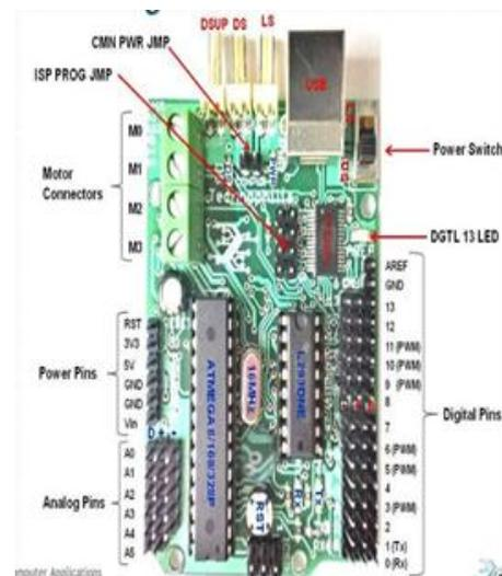
**Fig. 2:** Atmega 328p Micro Controller
