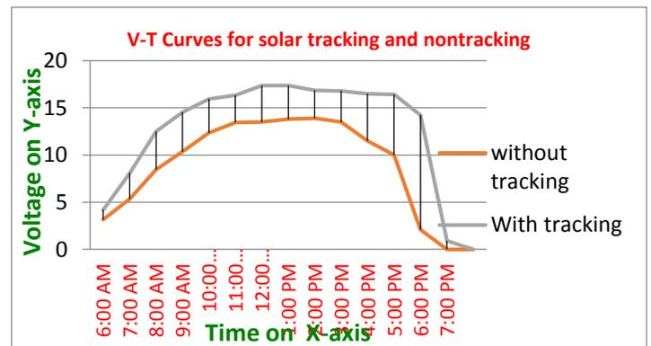
Fig. 9: Graph for voltage versus time for solar tracking and non-tracking.
