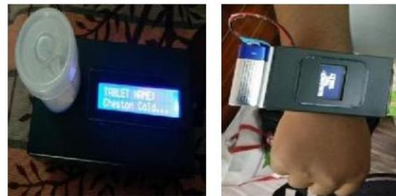
(a)Pill bottle with punched RFID tags. (b) Medifit
