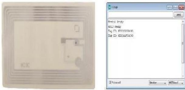
a) Passive RFID Tag b) RFID Tag read through Wearable
