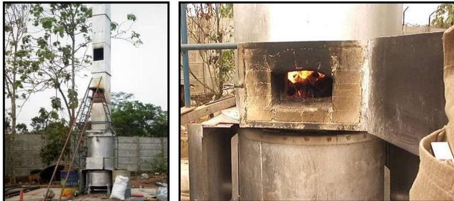
**Fig. 2:** Incinerating Process in Standing Furnace Incinerator (Incinerator Dapur Tegak)
