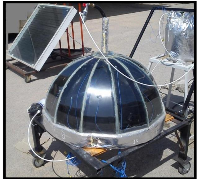
Fig. 1: A View of the Flat Plate and Semi-Spherical Solar Collectors.
