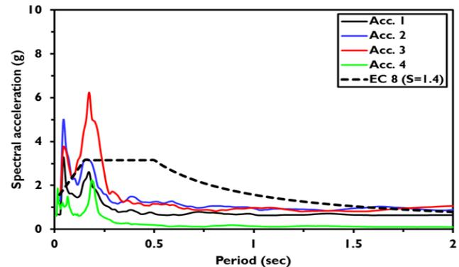
Fig. 12: Effect of Shaking on the Acceleration Response Spectra (Empty Test 1, 5% Structural Damping).
