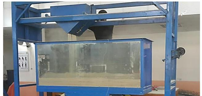
Fig. 3: The Mechanical Pluviator.
