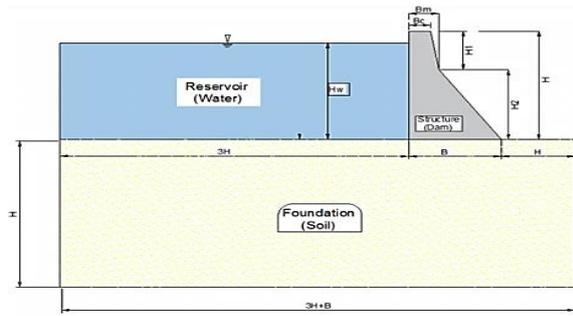
Fig. 1: The Geometric Dam Model.
