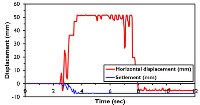
Fig. 15: Seismic Displacement and Settlement of the Dam Model (Test-2).
