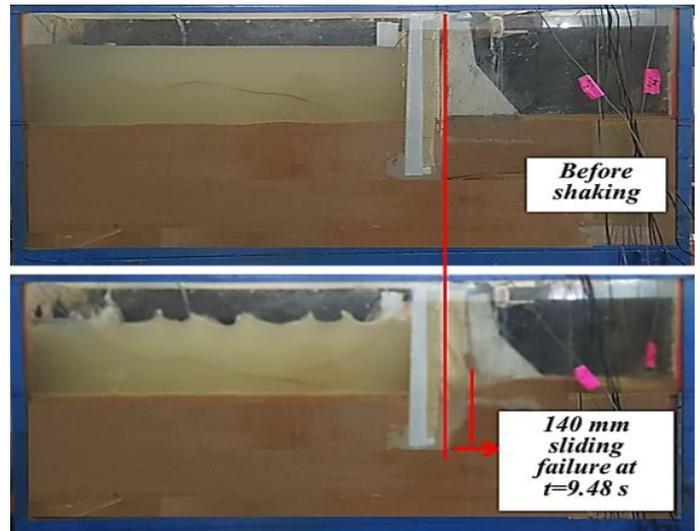
Fig. 19: The Sliding Failure of the Dam Model at the End of the Shaking.
