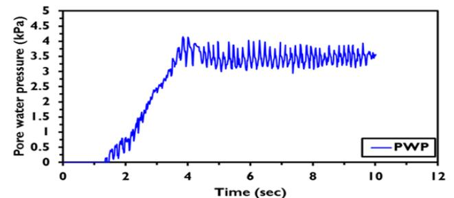
Fig. 16: The Measured Excess Pore Water Pressure (Test-1).
