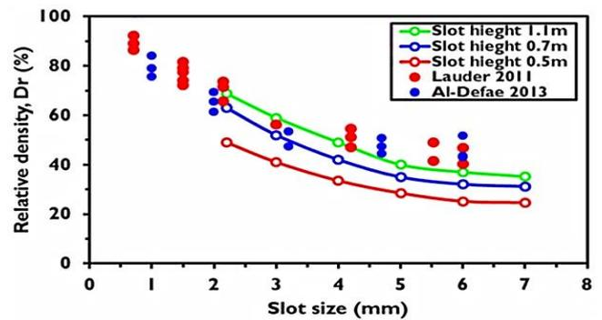
Fig. 4: Slot Size Correlation with Relative Density.
