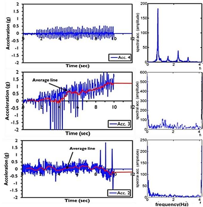
Fig. 11: Time Acceleration and Frequency Domain of Filled with Water Dam Model (I.E. Test 2).
