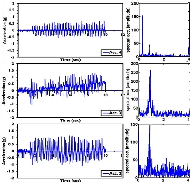
Fig. 10: Time Acceleration and Frequency Domain of Empty Dam Model (I.E. Test 1).
