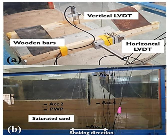
Fig. 8: Test 1; (A) LVDTs Positions and (B) Dam Model-Soil- Container.
