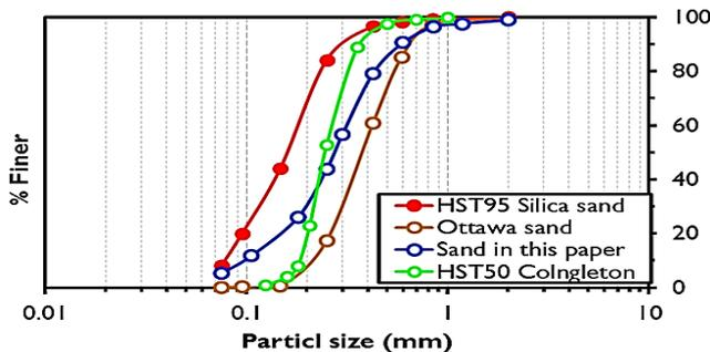
Fig. 2: The Grain Size Distribution of Used Sand.
