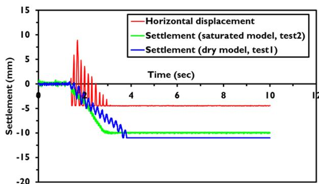
Fig. 14: The Measured Horizontal and Vertical Displacement for Saturated Soil-Dam System (Test-1).
