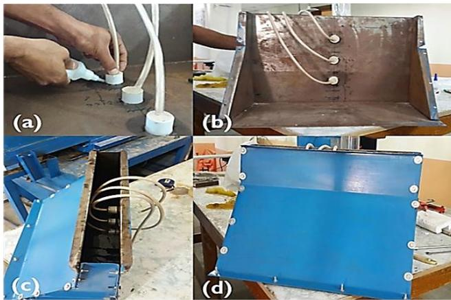
Fig. 6: Steel Framework and Sensor Holes Preparation.
