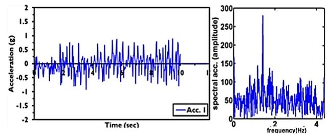
Fig. 9: Time Acceleration and Frequency Domain of Input Motion.
