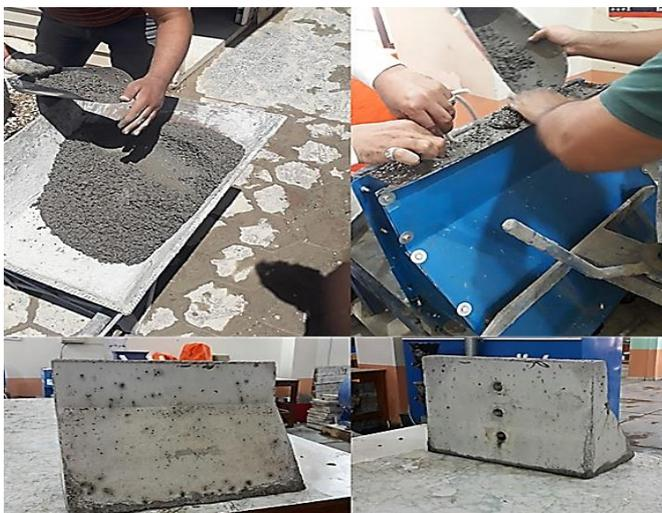
Fig. 7: Concrete Casting.
