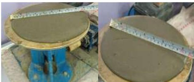
**Fig. 5:** Flowability of (a) unmodified mortar (b) mortar modified with 1 % PVA by mass of cement.
