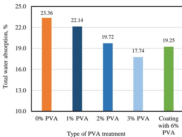
Fig. 4: Water absorption of the tested specimens
