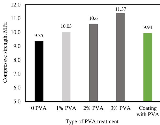
Fig. 3: Compressive strength of the tested specimens
