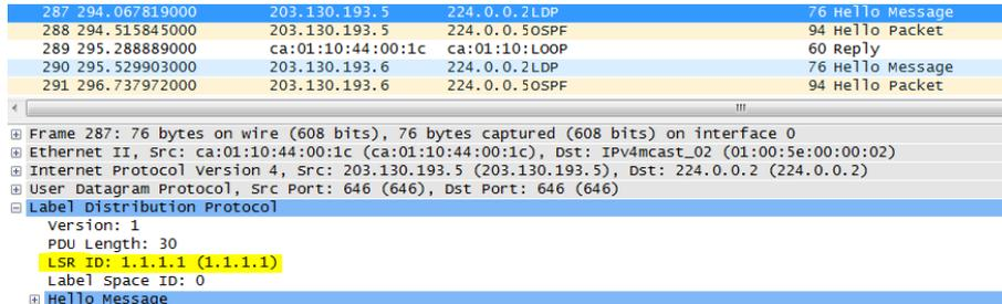
Fig 3: LDP packets passing through the router BTM-I
