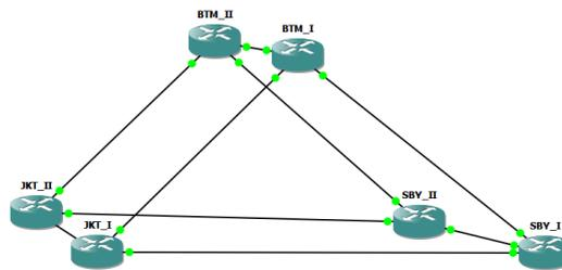
Fig 2: Topology system of MPLS for Telkom Architecture
