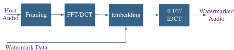
Fig 2: Watermark block diagram for embedding
