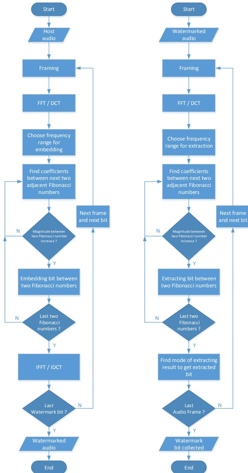
Fig 4a: Watermark embedding procedure, 4b Watermark extraction procedure
