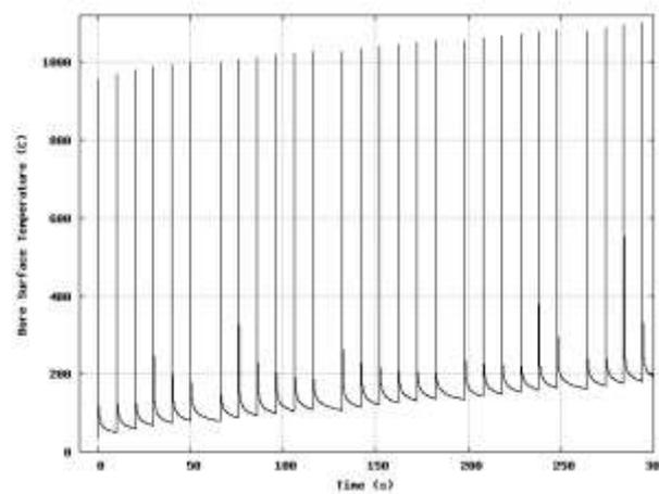
Fig. 6: Temperature history of bore surface with interval 10 seconds per shoot.
