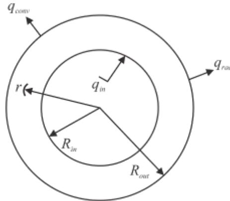
**Fig. 1:** Schematic diagram of a gun barrel with the illustration of heat transfer from inner to outer of bore surface.
