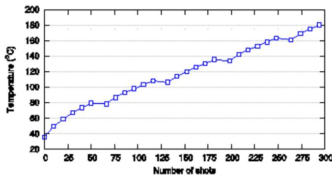
Fig. 5: Initial temperature of bore surface in each shot with interval 10 seconds per shot and rest time 6 seconds every 6 gun shots.
