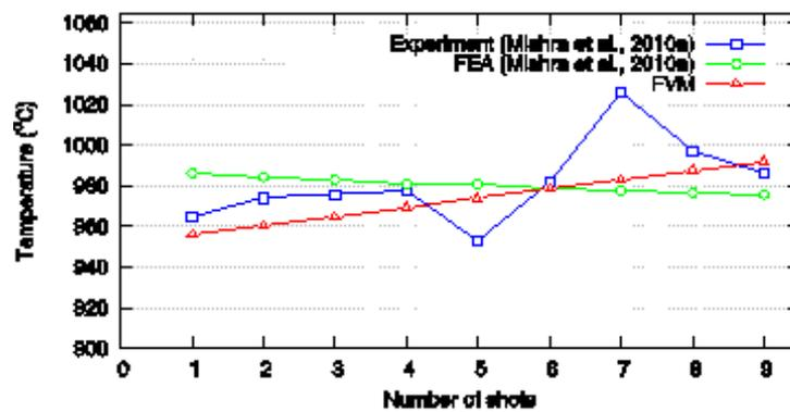
Fig. 4: Maximum temperature of bore surface in each shot (with interval 5 minutes per shot) using FVM against experimental data and FEA.
