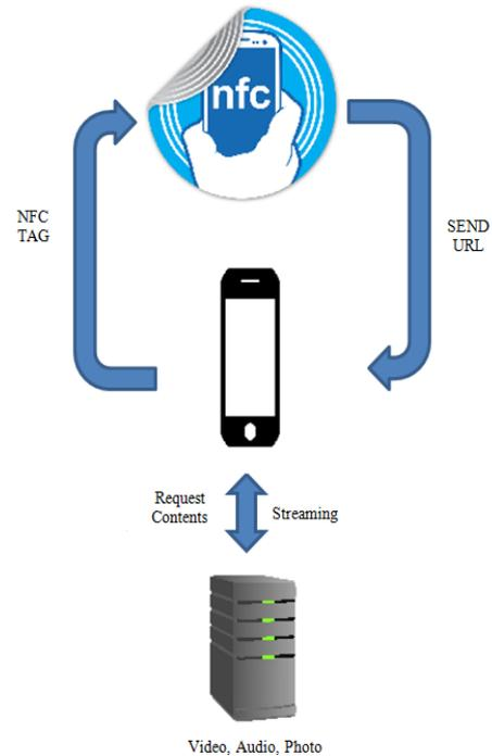
**Fig. 7:** Diagram of the NFC system-when an NFC equipped device is tagged to the NFC tag, prepared image, video and audio contents for the applying artifact are requested and then shown in the app
