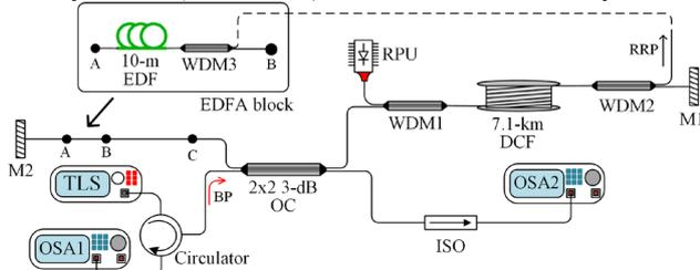
**Fig. 2:** Experimental setup: configuration-A, without EDFA block; configuration-B, with EDFA block. OSA: optical spectrum analyzer, TLS: tunable laser source, RPU: Raman pump unit, DCF: dispersion compensated fiber, OC: optical coupler, WDM: wavelength division multiplexer, EDF: erbium-doped fiber, M: Faraday mirror, BP: Brillouin pump, RRP: residual Raman pump, ISO: isolator.
