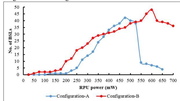
**Fig. 5:** Number of Brillouin Stokes lines with varying Raman pump intensity for configuration-A and configuration-B
