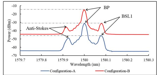
**Fig. 4:** Output spectrum of configuration-A and configuration-B at OSA3 with Raman pump intensity of 200-mW
