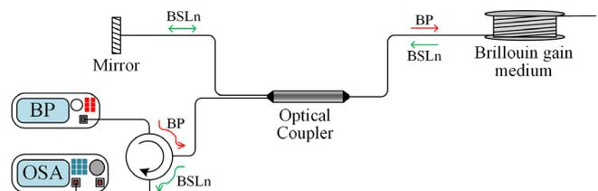
Fig. 1: Multi-wavelength Brillouin fiber laser setup.
