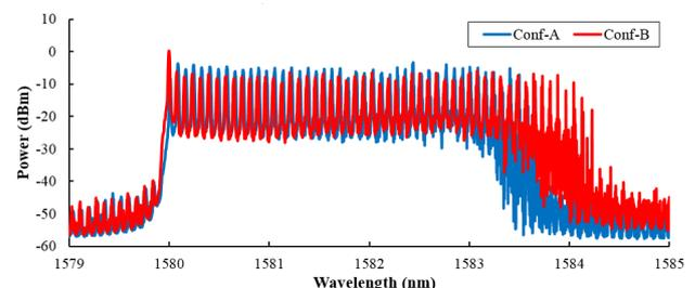
**Fig. 6:** Output spectrum of configuration-A and configuration-B at Raman pump intensity of 475 and 600-mW, respectively.
