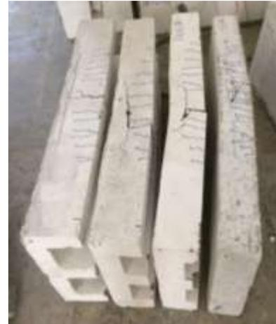
Plate 2: Failure Modes and Cracks Pattern
