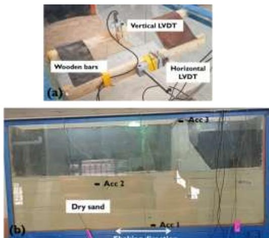
Fig. 9: Preliminary test; (a) LVDTs positions and (b) Dam model-soil-container
