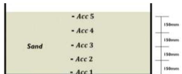
**Fig. 7:** Accelerometer distribution for the shaking table calibration
