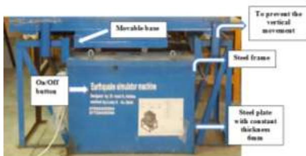
Fig. 2: The main parts of the shaking table.
