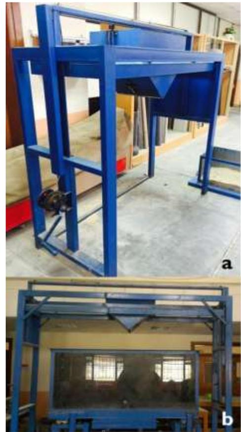
**Fig. 6:** Air pluviator technique; (a) The raining frame pluviator and (b) Pluviator and container
