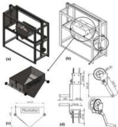
**Fig. 5:** (a) Pictorial view of mechanical pluviator; (b) Schematic view of pluviator; (c) V-shape container and (d) Mechanical chain and rope lever
