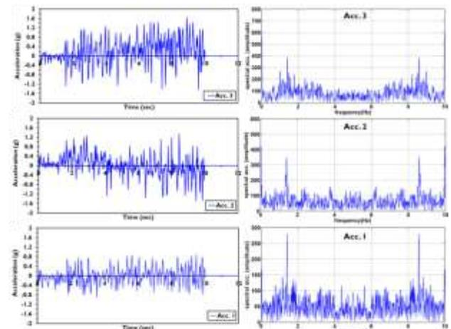
Fig. 10: The acceleration response of the dam-foundation system
