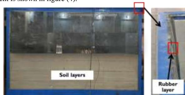
Fig. 3: The used container and the wave reflection rubber layer
