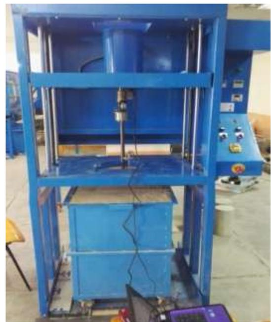
Fig. 2: Screw pile installation and loading machine with soil container and data collection via data logger
