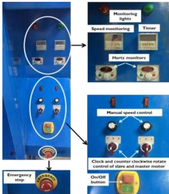
Fig. 3: Control board of the machine
