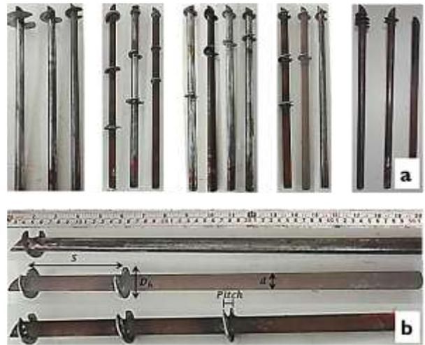
Fig. 7: Screw pile models; (a) all manufactured models and (b) dimensions and configurations
