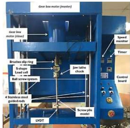
Fig. 1: Screw piles installation and loading apparatus
