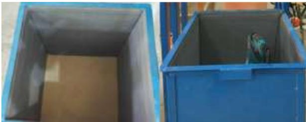
Fig. 6: The container used in the installation of screw pile models
