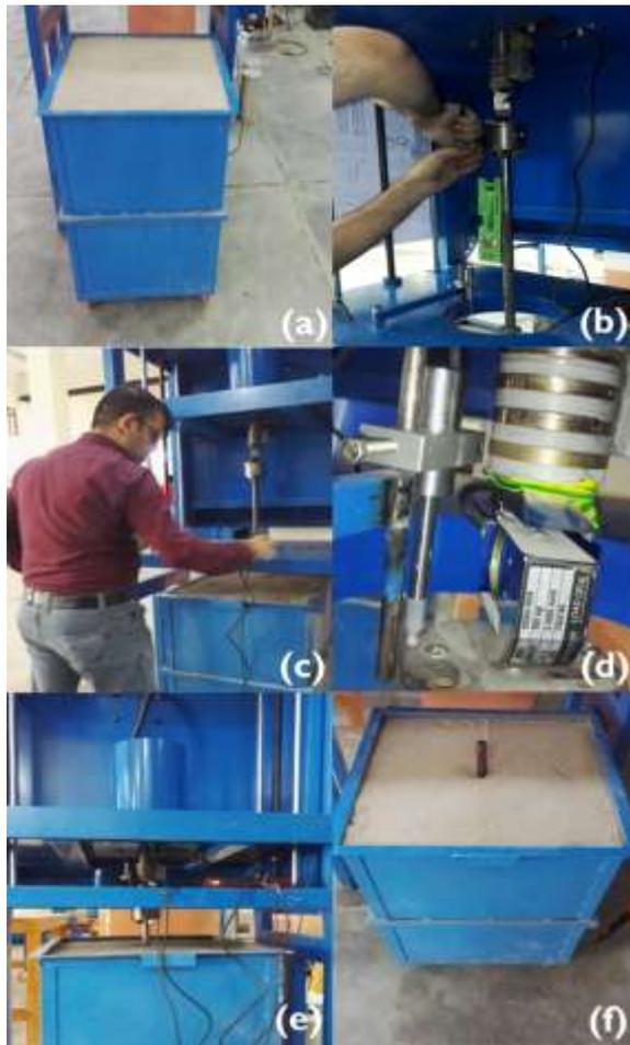
Fig. 8: Steps of screw pile model installation and testing
