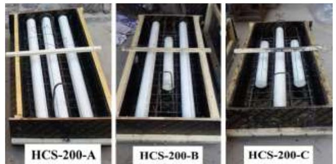
Fig. 4: Install Pipe and Steel Reinforcement in The Molds
