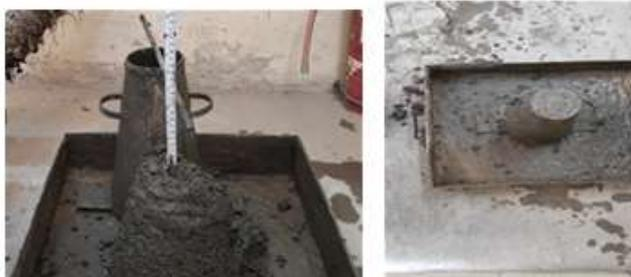
Fig. 8: Slump Test
