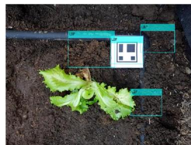
Fig. 13: Marker Detection Using LBP Features with Marker Detected Bounded by Cyan Box.
