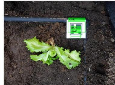
Fig. 11: Marker Detection Using Haar-Like Features with Marker Detected Bounded by Green Box.
