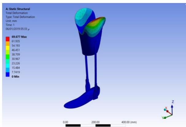
Fig. 16: Total Deformation.
