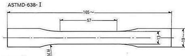
Fig. 1: The Dimensions of Tensile Sample According to ASTM D638.
