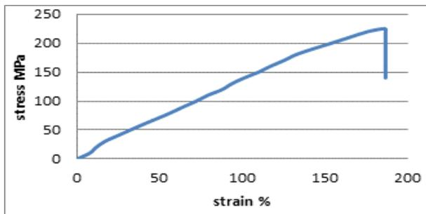
Fig. 6: Stress-Strain Curve for One Sample of Reinforced Composite with Fiber.
