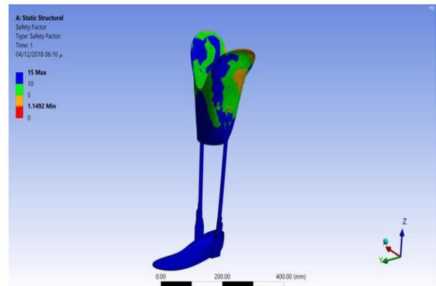
Fig. 17: The Safety Factor for Fatigue (Perlon).
