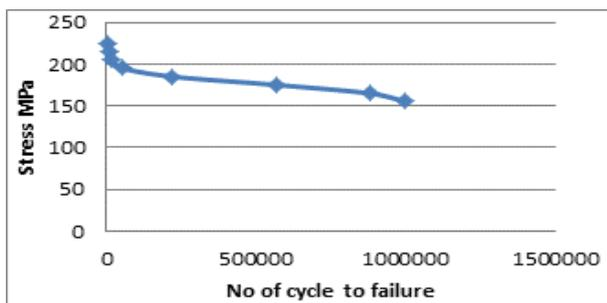
Fig. 7: S-N Curve for Composite Reinforcement with Fiber Glass.
