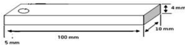
Fig. 2: Dimensions of Fatigue Samples.
