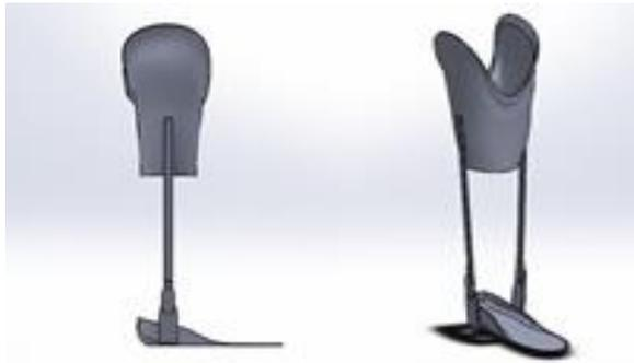
Fig. 5: 3-D Modeling of the Metal PTB
