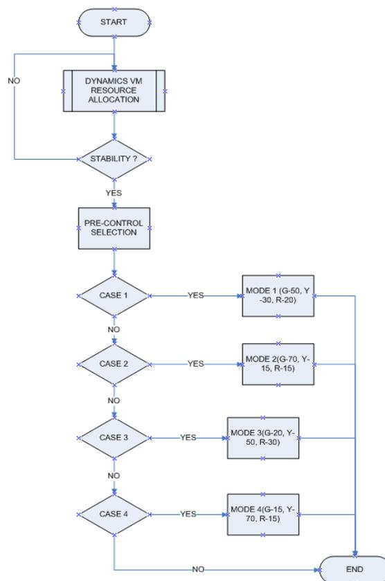
**Figure 6: Flow Chart of Stability Optimizer System**
