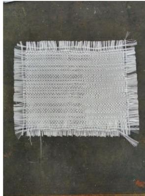
Fig. 1: E-glass fibers in mat form
