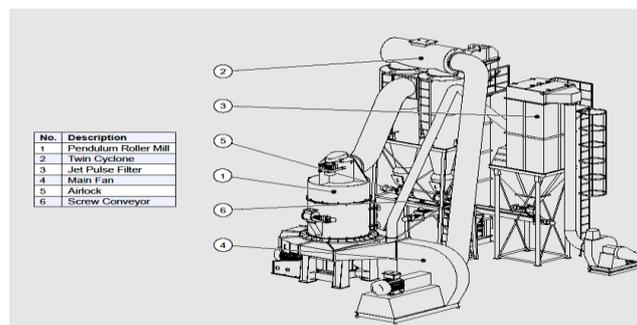
Fig. 2: Grinding plant layout
