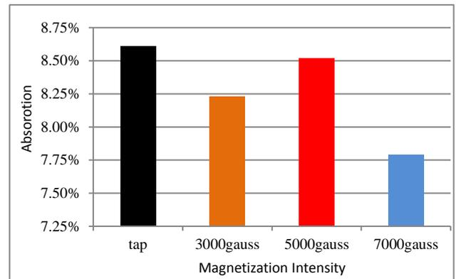
Fig. 10: Magnetized water effect on the absorption of concrete
