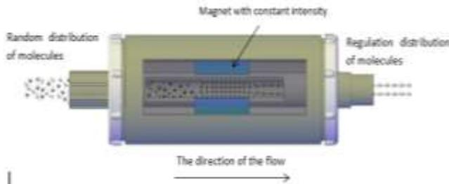
Fig. 1: Magnetic field effect on the distribution of water molecules
