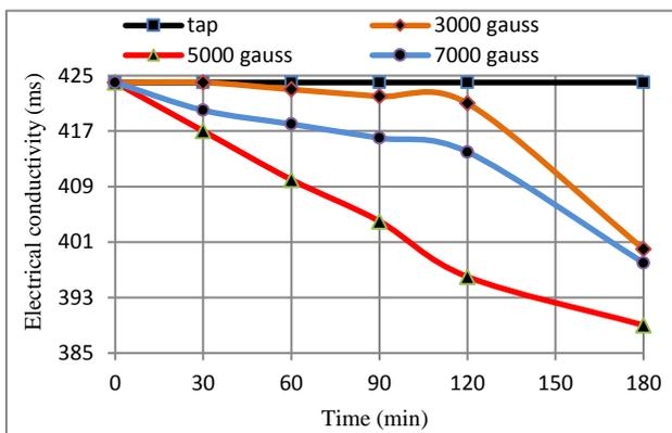
Fig. 7: Magnetic field effect on E.C. of water
