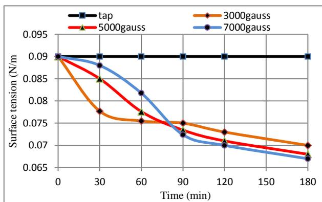
**Fig. 5:** Magnetic field effect on the surface tension of water
