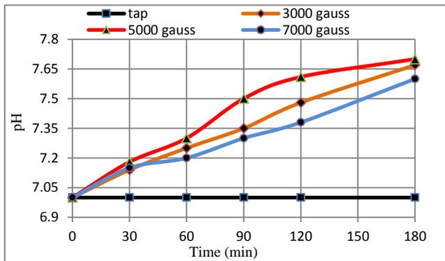
**Fig. 4:** Magnetic field effect on pH value of water
