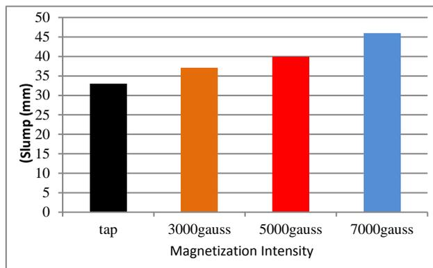
Fig. 9: Magnetized water effect on the slump of concrete
