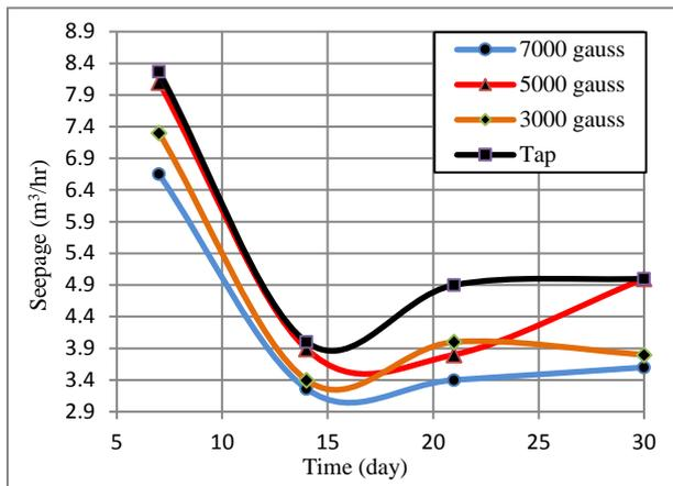
Fig. 11: Magnetized water effect on the seepage of concrete
