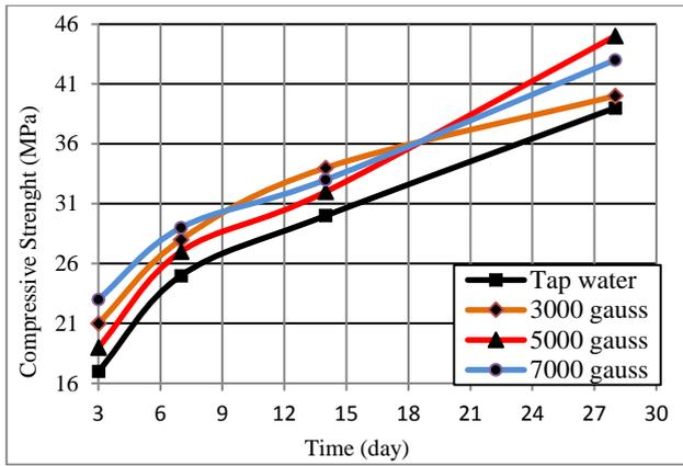
Fig. 8: Magnetized water effect on compressive strength of concrete
