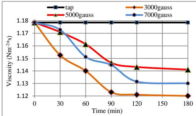
Fig. 6: Magnetic field effect on the viscosity of water
